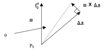
From the figure,  $\underline{\omega} \times \underline{\Delta a}$  represents a rotation of the end of  $\underline{\Delta a}$  about the vector  $\underline{\omega}$ ; at least, in the limit as  $t \rightarrow 0$ , or  $\underline{\Delta u} \rightarrow 0$ .
